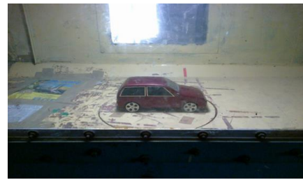
Figure.4. Model placed in the test section, view from the side glass
